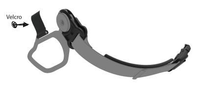
Mate this tab with supplied adhesive backed Velcro to eliminate rotation of the Cutaway handle
